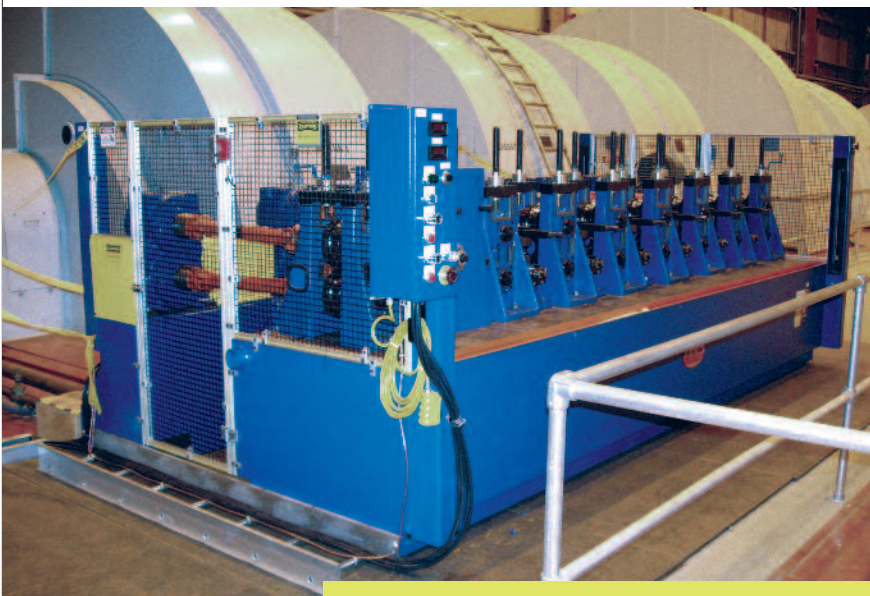
Tube-reducing machines are one of many types of equipment custom-made at Formtek.
